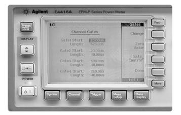
Versatile user interface displays up to four time gates and lengths in a single measurement setup. This menu is accessed using the CHANNEL hardkey.
